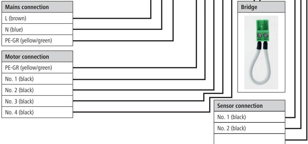
Figure 7: Circuit board connection diagram with capacitor - Uno
